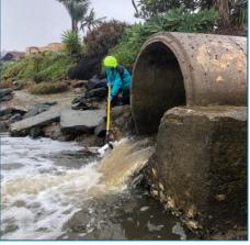
Sample collection of stormwater runoff
